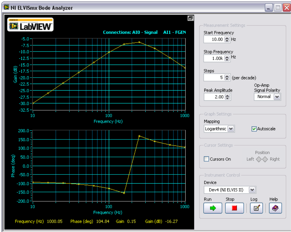
Figure E4-2. Frequency Response Verification of Real-World Circuitry
