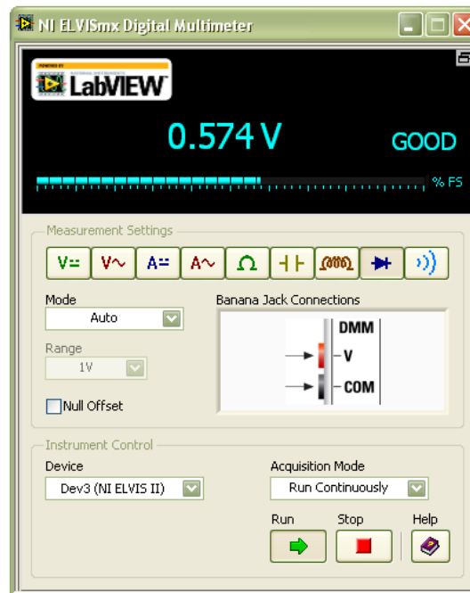
Figure 3. Forward-biased Diode Reading
